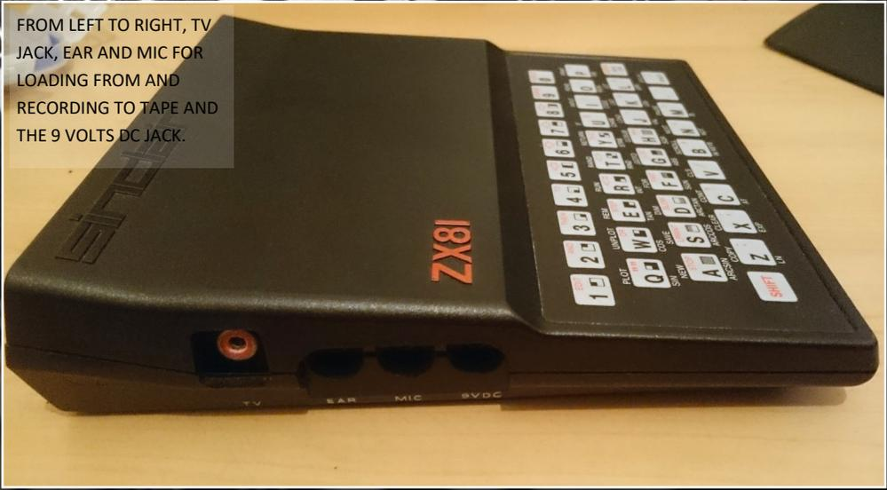
FROM LEFT TO RIGHT, TV JACK, EAR AND MIC FOR LOADING FROM AND RECORDING TO TAPE AND THE 9 VOLTS DC JACK.
